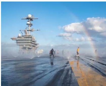
Sailors test of the countermeasure wash-down system on the flight deck of the aircraft carrier USS John C. Stennis in the Atlantic Ocean.
