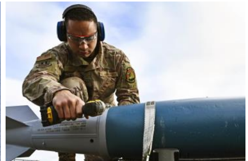
Air Force Staff Sgt. Tomas Gonzales screws fins onto a BDU-50 practice munition at Royal Air Force Fairford, England, Oct. 16, 2019.
